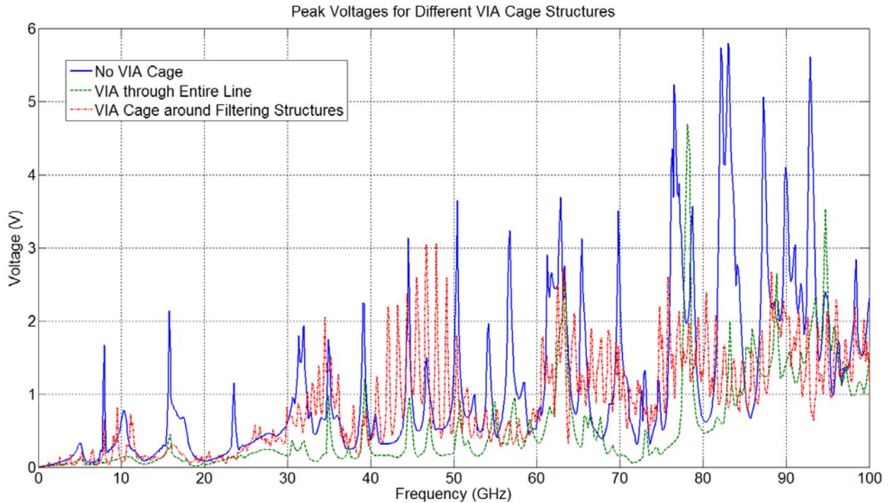
**Figure 19. Parallel Plate Voltages for the different VIA cage options**
