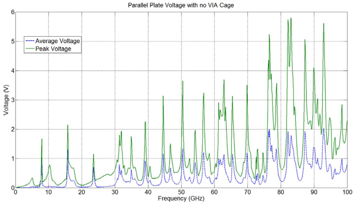
**Figure 16. Parallel Plate Voltage for the Stripline CRLH Filter**
