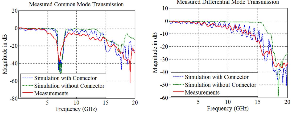
**Figure 4. Measured vs Simulation showing the more accurate model when the connector model is included.**
