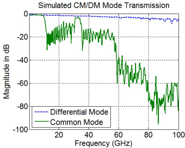
**Figure 13. Common Mode vs Differential Mode Transmission**
