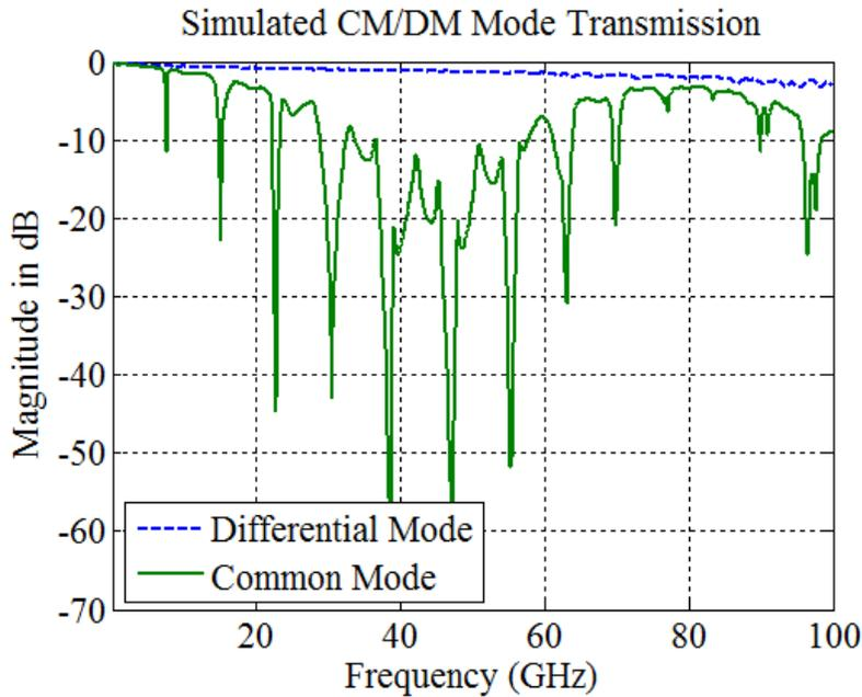
**Figure 10. Common Mode vs Differential Mode Transmission**
