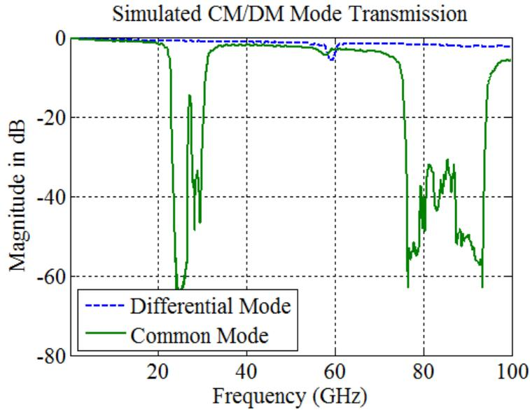
**Figure 12. Common Mode vs Differential Mode Transmission**
