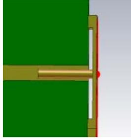
**Figure 6. Top view of SMA connector model**
