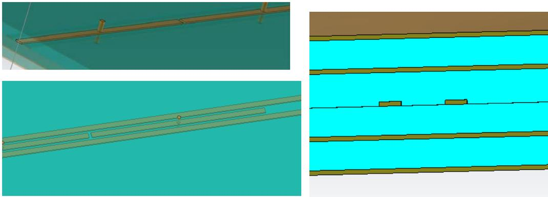
**Figure 14. CST Model of Stripline Structure with CRLH based CM Filter**
