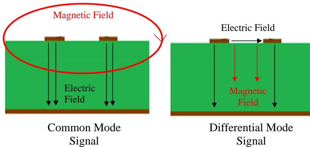
**Figure 1. Common Mode vs Differential Mode Signals showing the fields in a microstrip**
