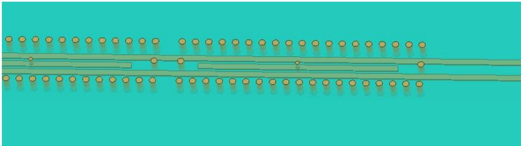
**Figure 18. VIA fence implemented around individual filtering structures**
