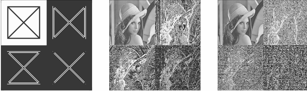
Figure 13: Detection of borders with the wavelet transform. The dark zones have been enhanced. Left to right: Original image and wavelet transform with one level of resolution.
