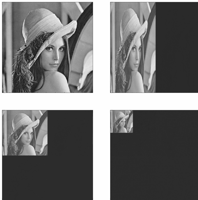
Figure 12: Wavelet transform of an image using the MRA of Daubechies with four vanishing moments. Left to right and top to bottom: Original image, wavelet transform by rows, and wavelet transforms with one and two levels of resolution.
