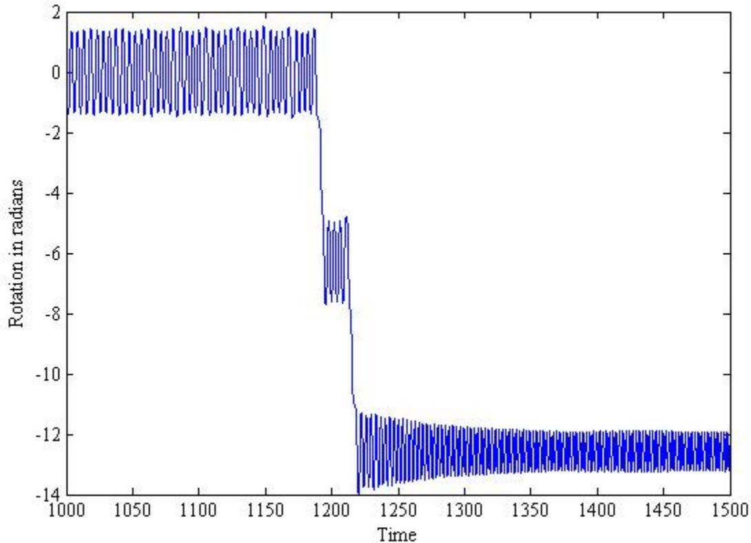
Figure 3.4-4—The Tacoma Narrows deck flipping over completely
