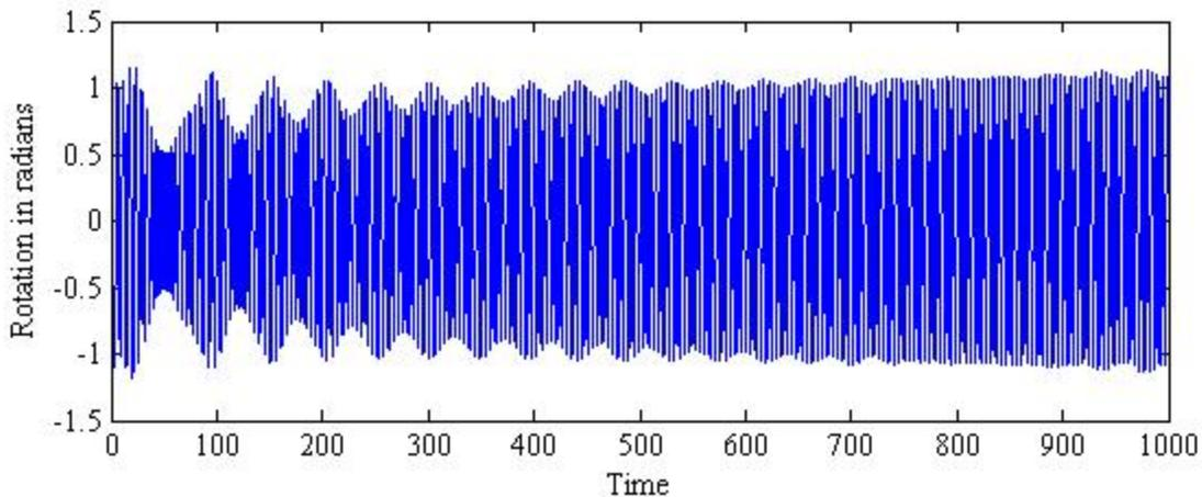
Figure 3.4-1—The bridge response due to weakening cables with a reduction factor of  $w = 1,000$  and rate factor of  $b = 1.00$
