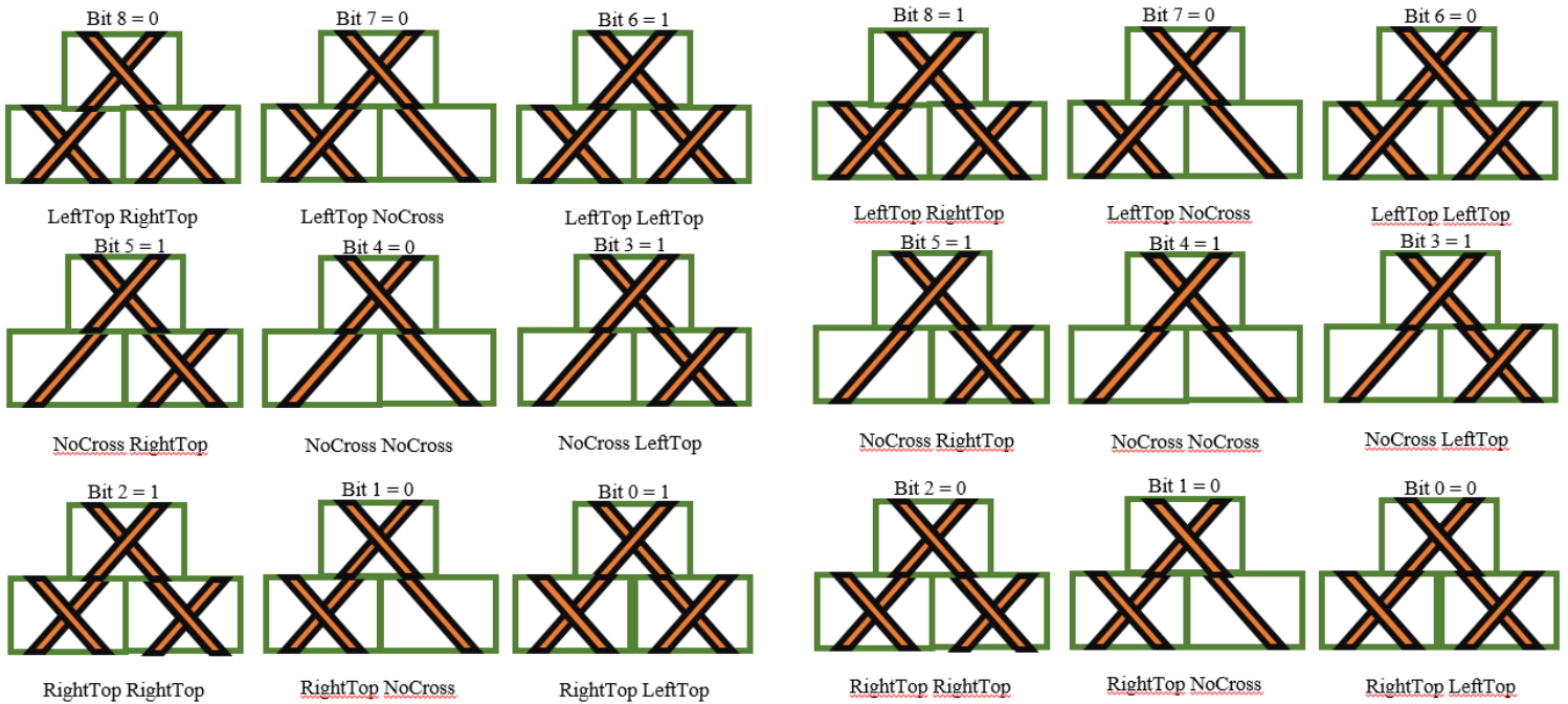
Figure 5.b: Sample conversion of crossing rule (the left set is the original crossing rule and the right set is the mirrored crossing rule).
