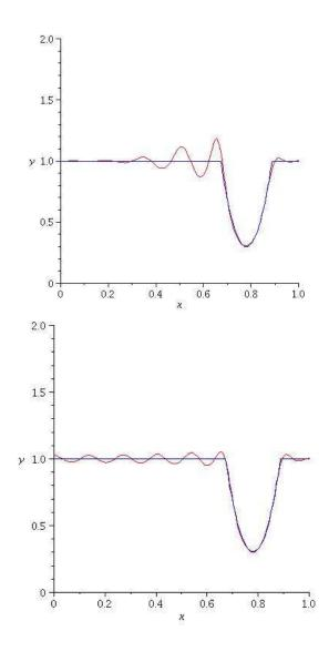
Example 2.2.1 illustrates how computational error affects the reconstruction process. This example reconstructed  $\gamma$  using a 14-term Fourier approximation. Adding higher order terms in this case introduces error that renders the reconstruction useless. The reason for the instability in the recovery of higher order terms can be seen in equation (8). The reconstruction algorithm solves for the  $c_j(t)$ 's from boundary data. In terms of the  $c_j(t)$ 's then, the  $f_j$ 's are:
