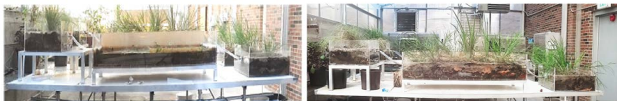
Figure 2: Subsurface (SSF) wetland system (left) and free water surface (FWS) wetland system (Mueller Price, 2015)
