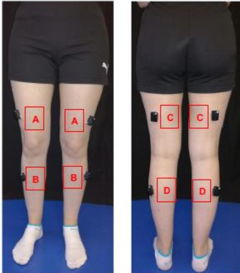
Figure 2.2: Moreira et al. [2] sEMG Sensor Placement
