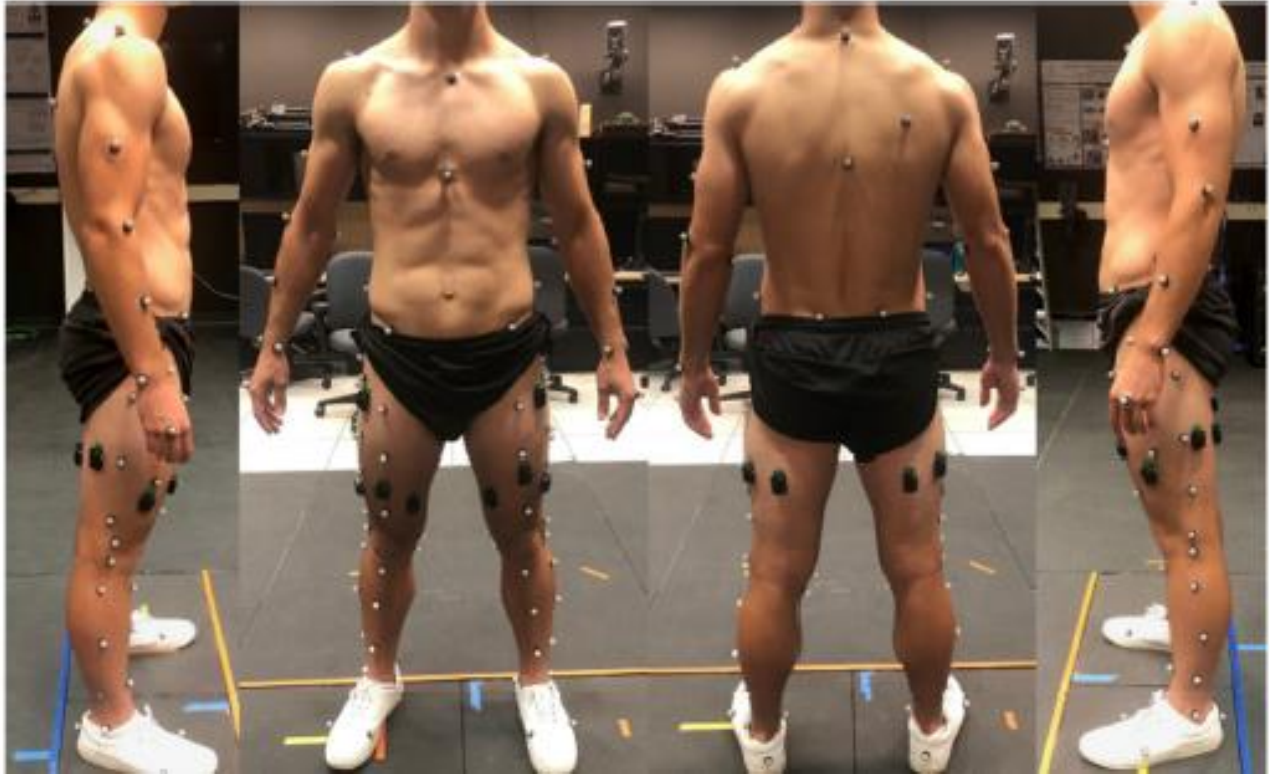
Figure 2.1: Coker et al. [2] sEMG Sensor and Retroreflective Marker Placement
