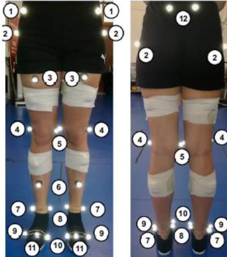
Figure 2.3: Moreira et al.[2] Retroreflective Sensor Placement
