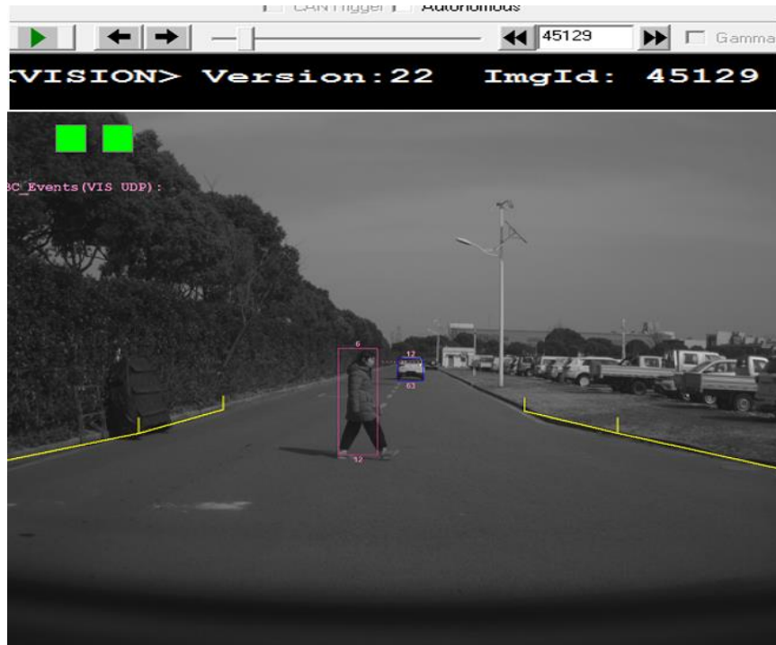
Figure 2. The Detection of a Pedestrian and a Vehicle by the ADAS Camera.
