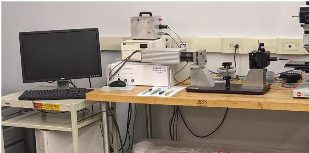
Figure 3.3 - The ellipsometer used in from the M.I.N.D.s facility. It has a stage for the sample and an adjustable source and receiver that can be manually adjusted with the stage.
