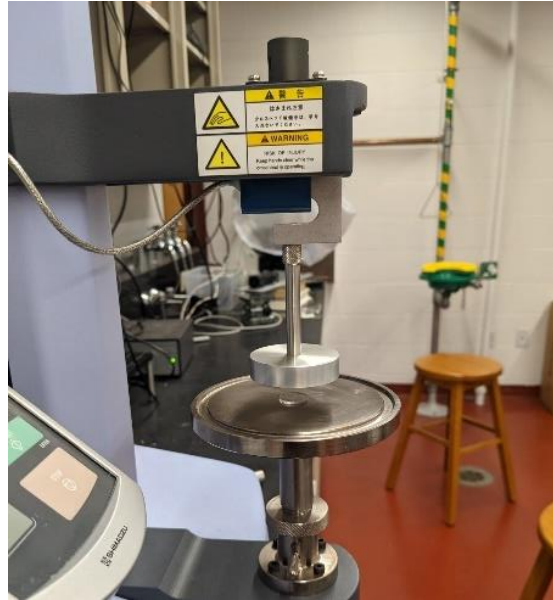
Figure 3.1 - The Shimadzu Trapezium X texture analyzer pictured with the attachment used for compression testing.
