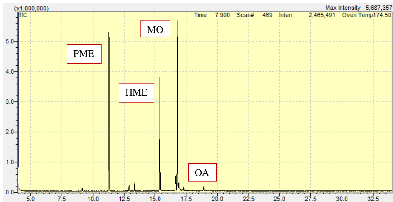
Figure 6.2.12: Example of a chromatograph of an unknown studied at an injection temperature of 300°C that has random artifact peaks that are not usually seen between 12.5 min and 13.5 min. They are most likely degradation products of the TMS derivatives or methyl oleate.
