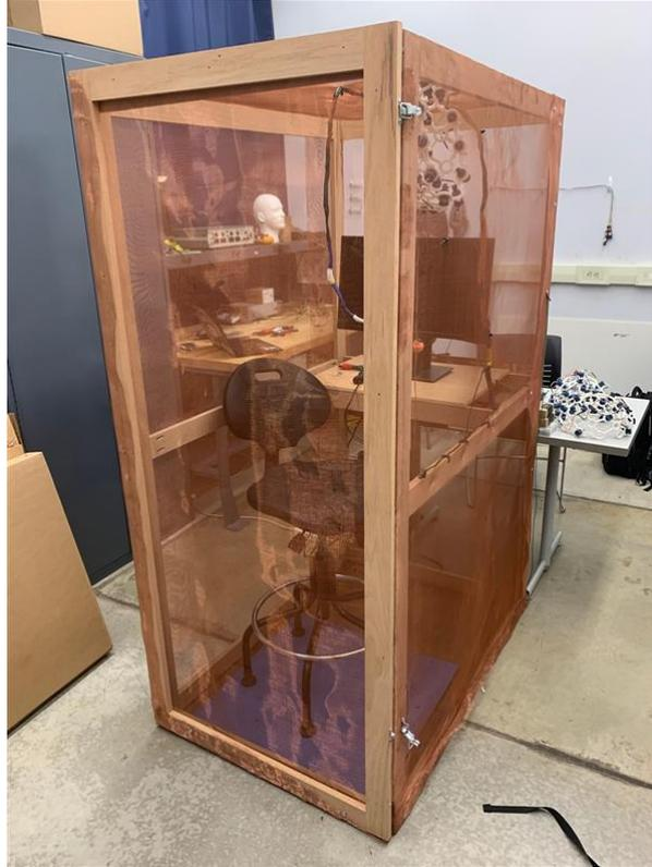
**Figure 7.** Faraday Cage Setup with monitor system in the BCI research lab. Subjects would have sat in this enclosure while wearing one of the two headsets seen in the photo. The RSVP protocol would have been implemented on the screen in the enclosure with data live streaming to researchers in the room.
