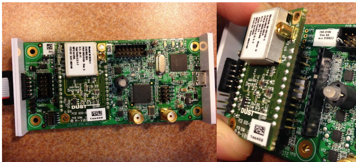
Figure 63 Steps to open the enclosed circuit box and plug the LTP5900-WHM module to the ESP socket.
