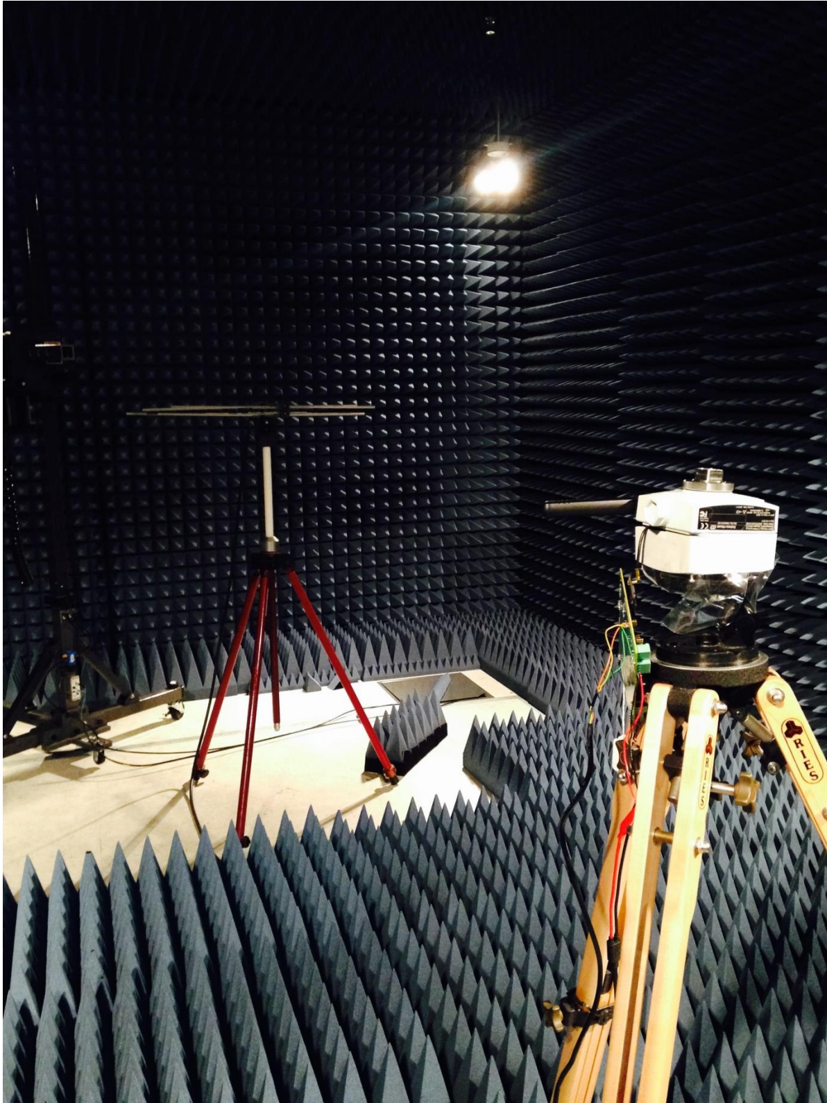
Figure 30 Radiated power measurement setup inside an anechoic chamber
