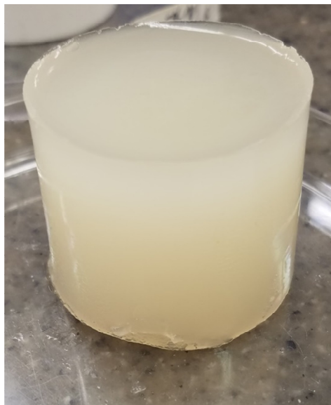
Figure 15. Phase separation in blend samples at pH 5 using the third gelatin batch.
