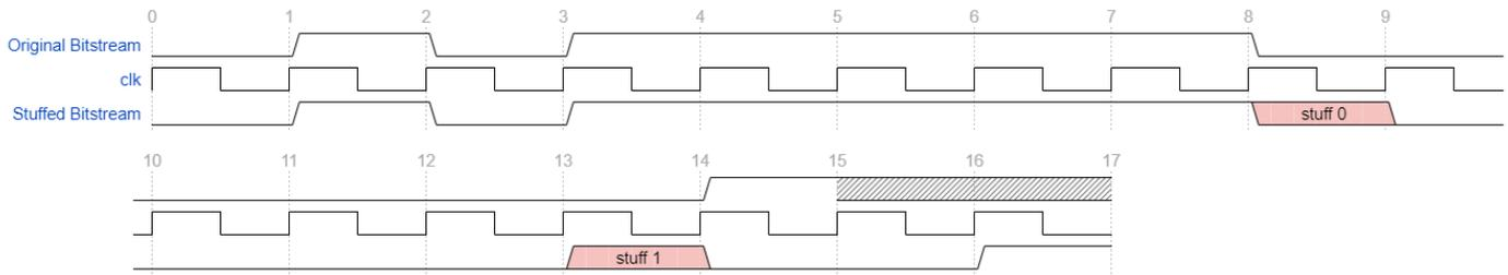
Figure 10 CAN Bit Stuffing Scheme
