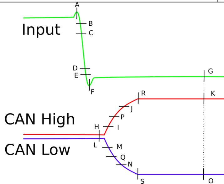
Figure 21 MCP2551 Dominant Driver Delay Waveform
