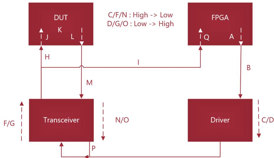
Figure 22 Labeled Signal Delay Path
