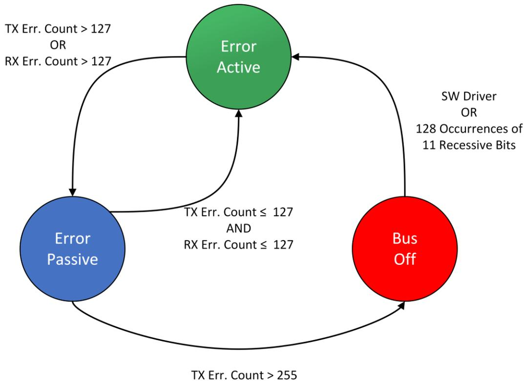
Figure 11 CAN Error State Machine
