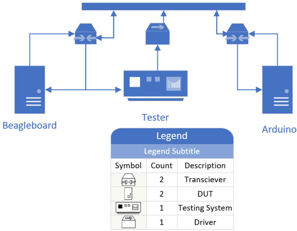
Figure 18 Design for Verification Test Bench
