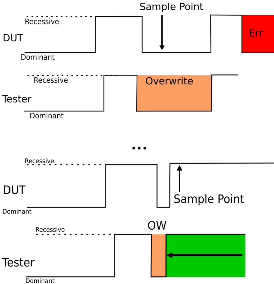
Figure 14 Diagram of Beginning Aligned Sample Point Detection
