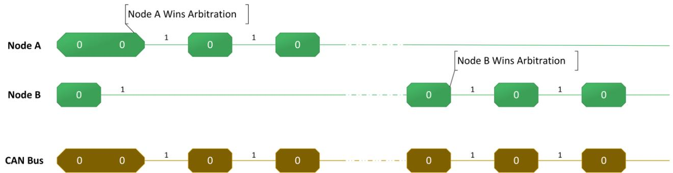
Figure 8 Two Nodes Arbitrating for Bus Control
