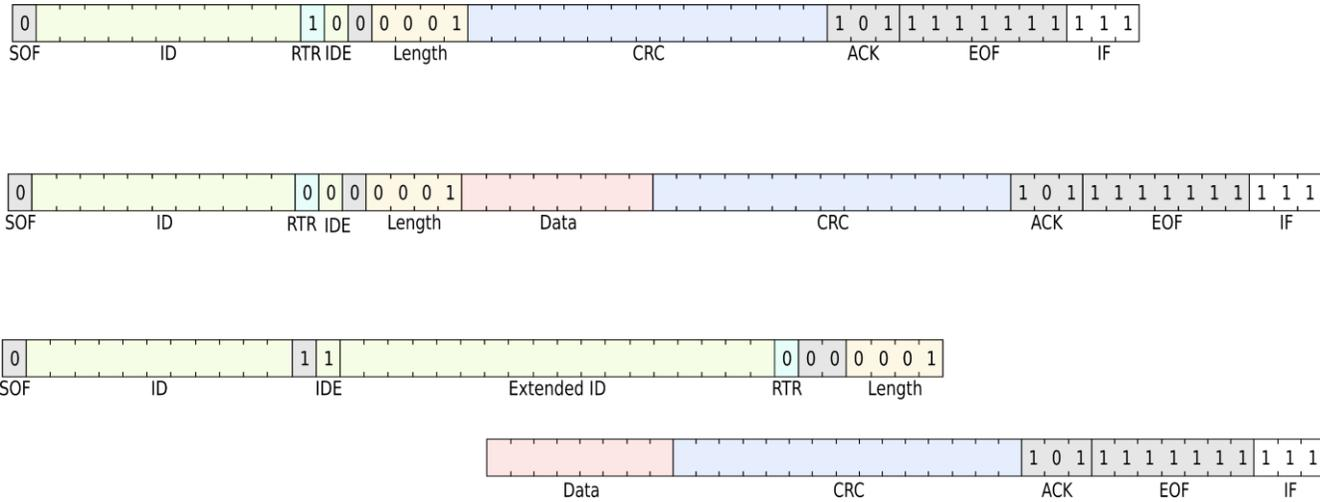
Figure 2 Comparison of CAN Data Frames
