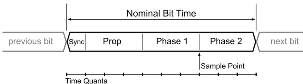
Figure 9: CAN Bit Timing Diagram
