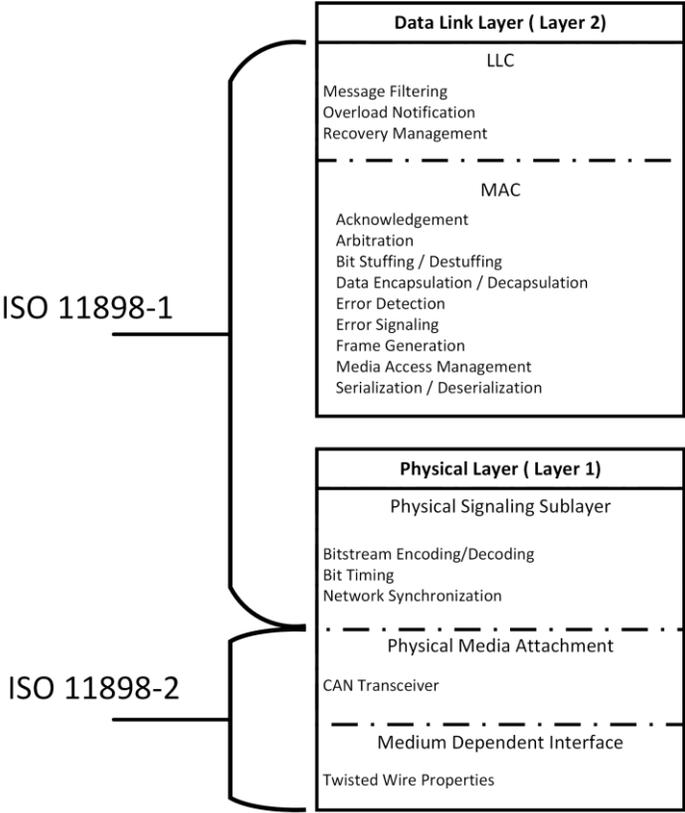
Figure 1 OSI Layout of Controller Area Network[2]
