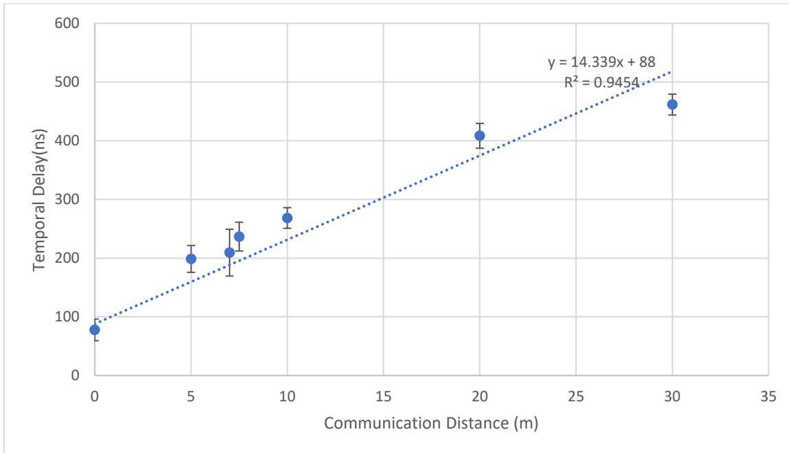
Figure 35 Experiment 3 Temporal Delay vs. Transmission Line Length
