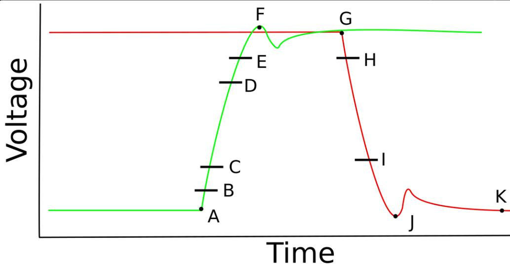
Figure 20 MCP2551 Receiver Dominant to Recessive Delay Waveform
