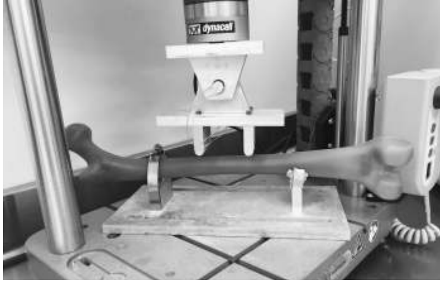
Figure 3.1 Intact composite bone in lateral in tension loading set-up with rotation constrained by a clamp in the proximal end and a custom mold on the distal end
