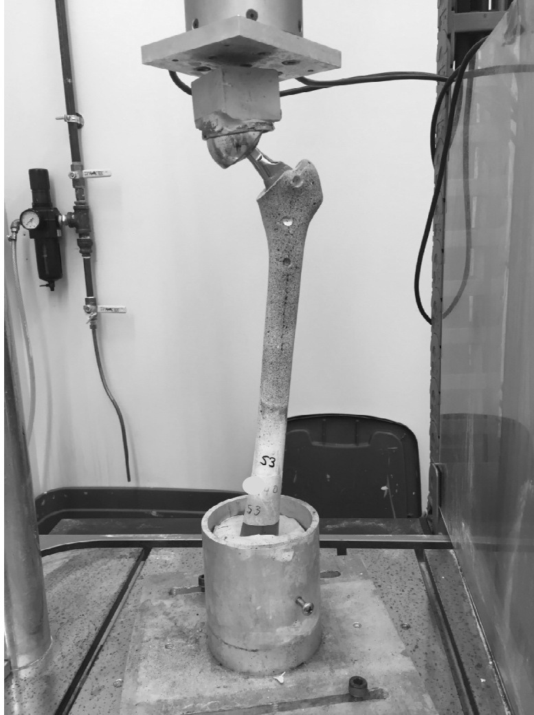
Figure 3.3 Implanted composite femur in axial stiffness loading set-up
