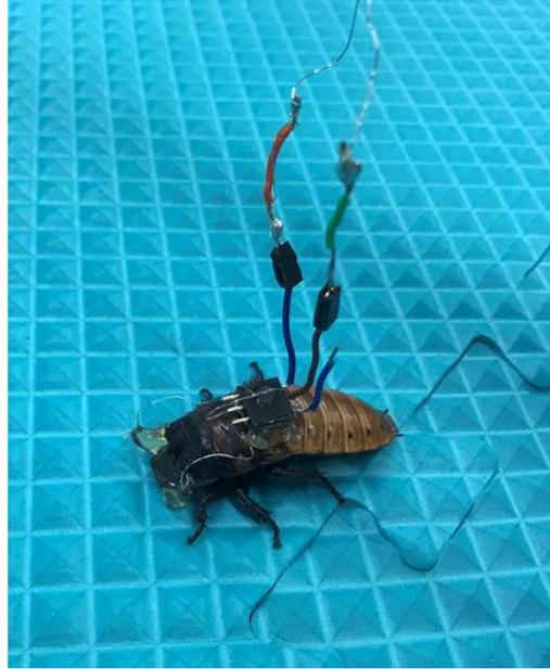
**Figure 12.** A subject hooked up to the pulse generator with thin platinum wires, which minimizes the amount of tension placed on the subject. The green wire denotes ground, and the orange wire denotes the wire that provides the stimulus to the right antenna.
