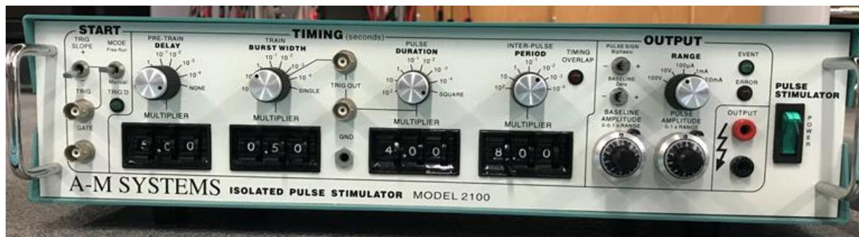
Figure 11. The Isolated Pulse Stimulator Model 2100 (A-M Systems) was used to create biphasic pulse trains.
