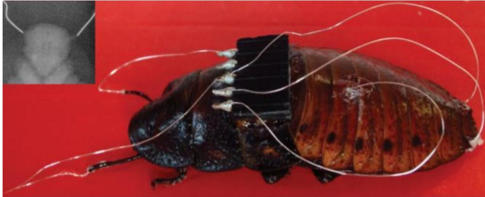
**Figure 5.** A Madagascar Hissing Cockroach biobot with electrodes implanted in its antennae, cerci, and abdomen [5].
