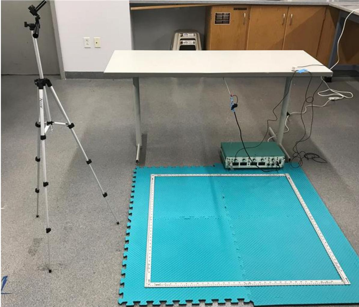
**Figure 13.** The experimental set-up, showing the function generator, the smartphone tripod, and the blue mat where the subject received stimulation.
