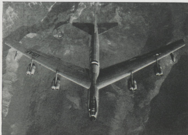
BOEING B-52 — Eight J-57 engines, mounted in pairs, power this all-jet, heavy Air Force bomber.
