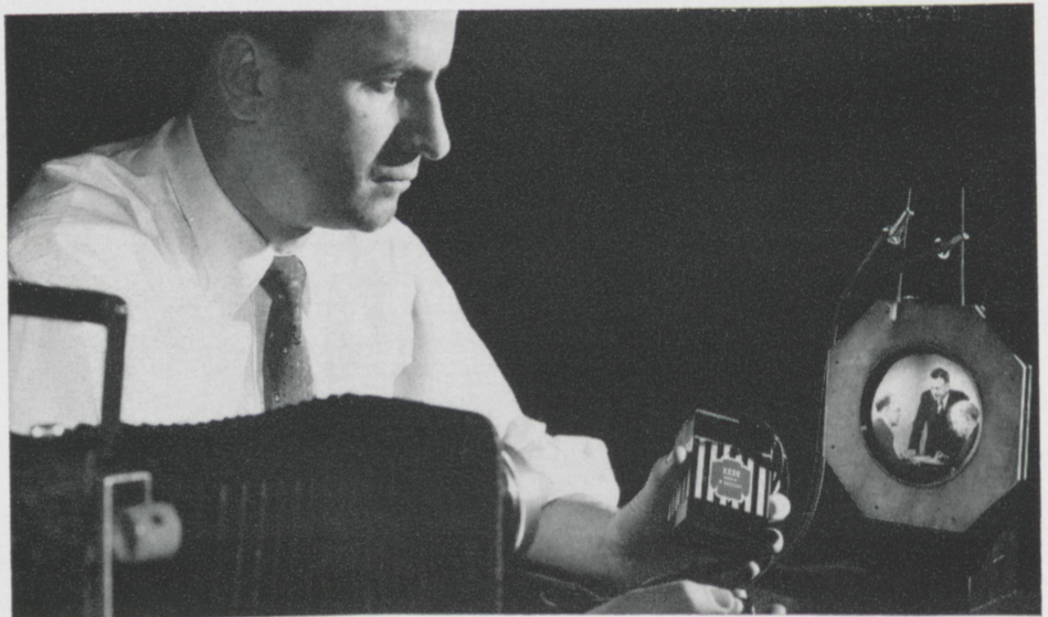
DIRECT AMPLIFICATION of light that is independent of electronic tubes occurs only when electroluminescence is "triggered" by light striking an experimental phosphor screen. Cut courtesy General Electric Company.
