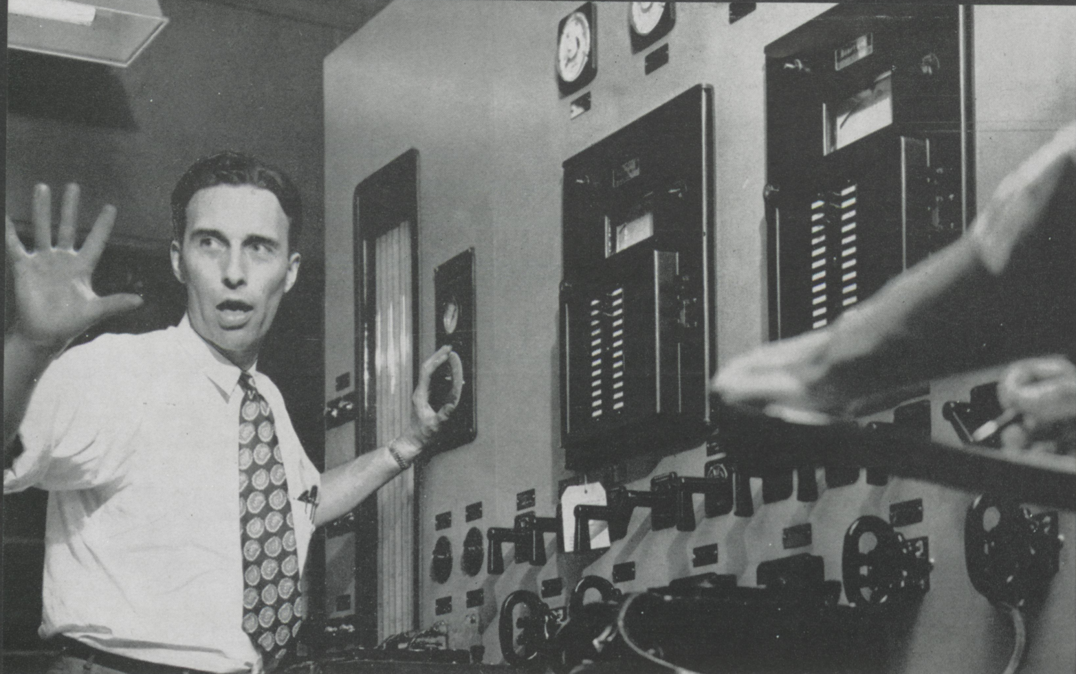
"POWER OFF!" Test operations are directed from this central control room, where special measuring instruments greatly speed up the collection of pump performance data. That's one way Worthington products are made more reliable by using . . .
