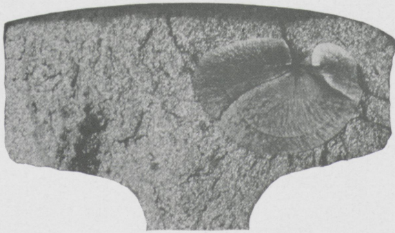
Two typical views of fissures. The one on the right would have broken in a very short time.
