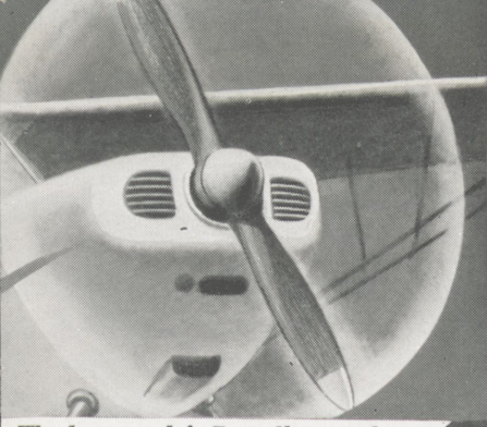
Wonder woods! Propellers and many aircraft parts are produced with "Bakelite" resin-bonded molded plywoods.
