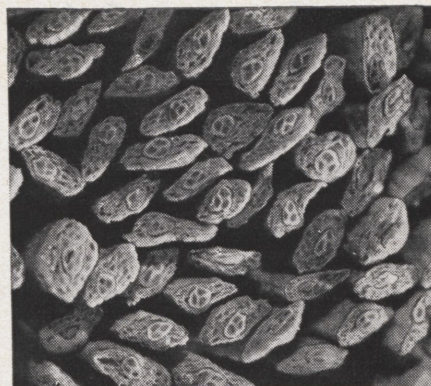
CROSS-SECTION of the new mop yarn. Each cotton fiber strand is jacketed with cellulose sponge material.
