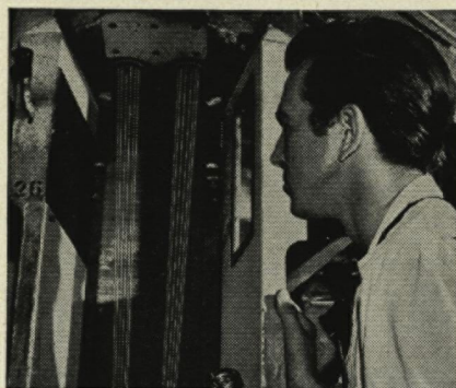
Inspecting nylon filaments during manufacture. They are made by extruding molten polymer through spinnerets under pressure.
