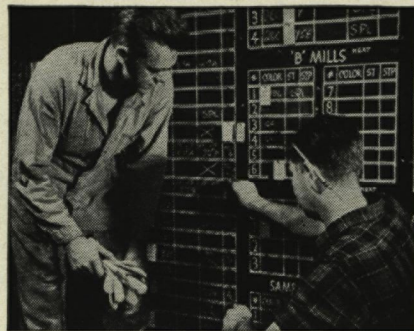
Operator and foreman check raw materials on a production control board which records every operation in a Du Pont plant.
