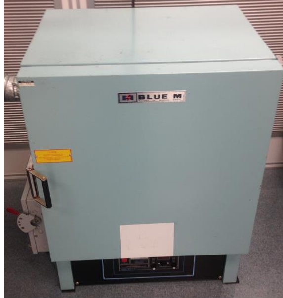
Figure 3.20: Oven used for oxidizing samples
