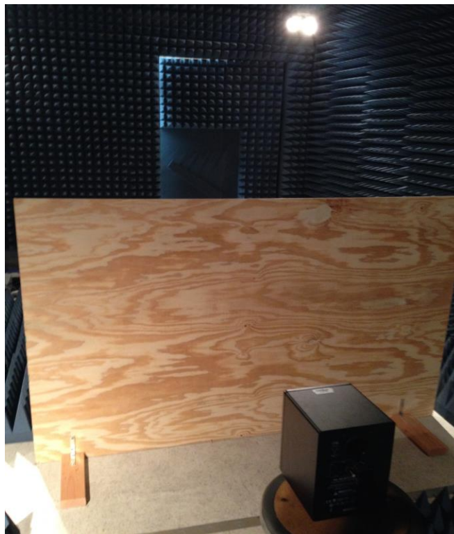
Figure C.2. The source side of the anechoic chamber after barrier insertion
