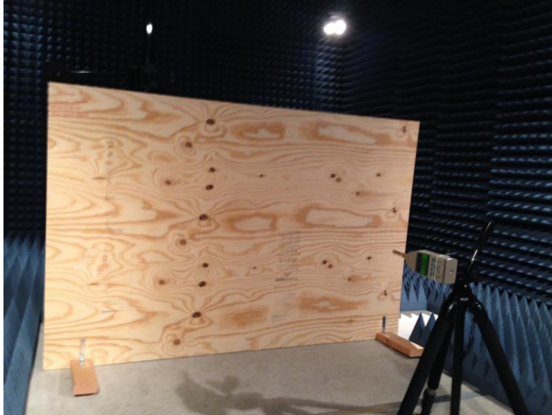
Figure C.1. The receiver side of the anechoic chamber after barrier insertion
