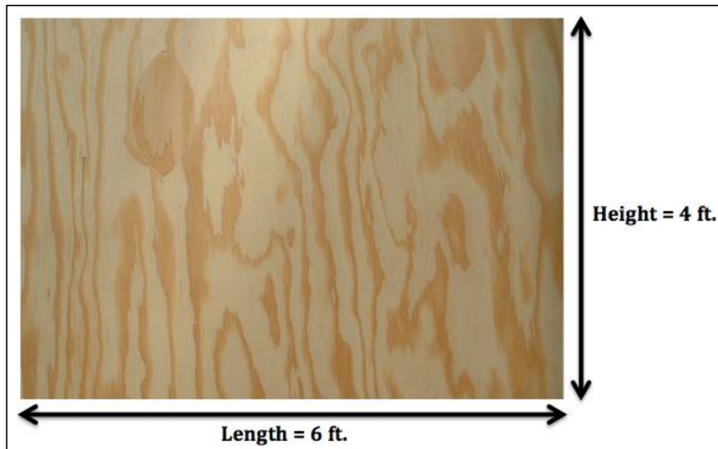
Figure 4.3. 4 × 6 ft. Plywood sheet used as the sound barrier with a 0.5 in. thickness
