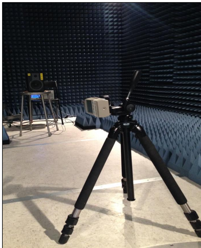
Figure 4.9. Setup used for making SPL measurements before barrier insertion
